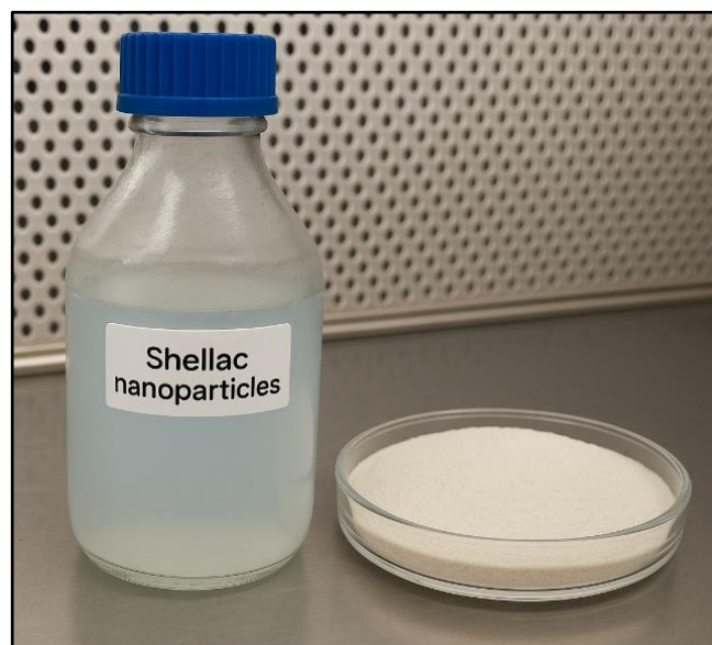
Shellac nanoparticles (Colloidal suspension and the dried powder)
