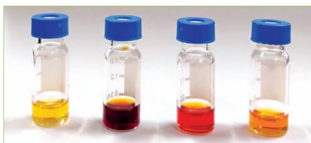
Lemongrass EO extracted by different methods : (a) hydrodistillation, (b) ChCl: Urea, (c) ChCl: oxalic acid, (d) ChCl: Citric acid
