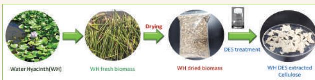
Cellulose extraction from water hyacinth using DES extraction
