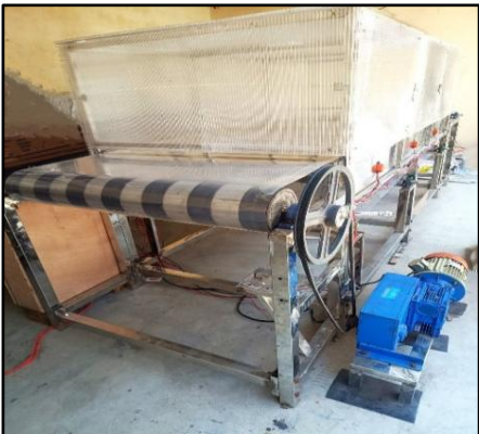
Fig 2. Continuous type Refractance Window Dryer
