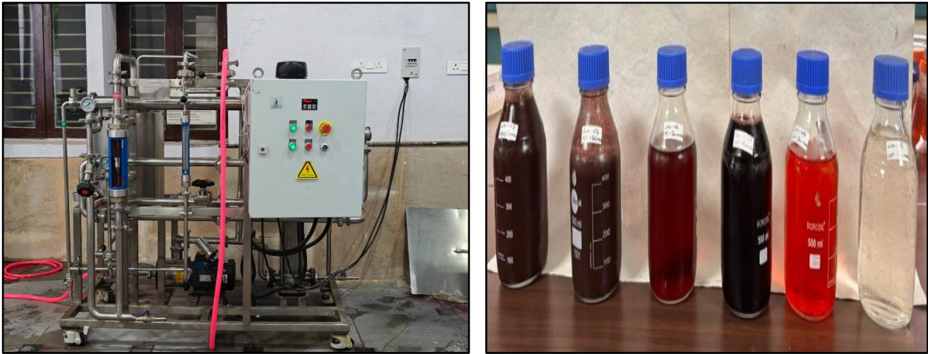
Fig 6 (a) Membrane Separation of Lac Dye from Wash water, (b) different fractions from Feed, Permeate and Retention from MF, UF and NF
